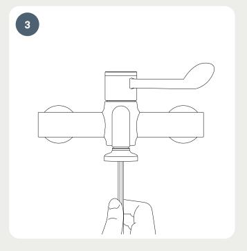
Locate the pin hole on the adapter.
