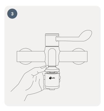
Install the product directly from the packaging and ensure that the filter does not come into contact with sources for contamination before being installed. Push the filter into the adapter until it is depressed fully with an audible 'click'.
