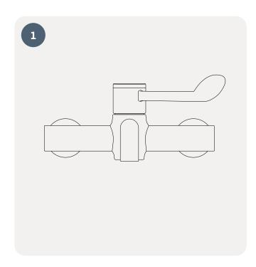
Prepare the outlet for installation of the adapter by removing any existing inserts such as flow straighteners or aerators. Check the tap thread for signs of damage and ensure it is clean and free from limescale before installing the Adapter.
