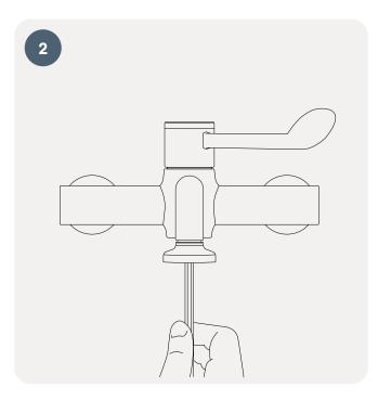
Mount the adapter to the outlet using a 10mm hex key to achieve a watertight seal.
