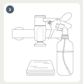
Prepare the adapter for the Bypass Sampler by ensuring it is clean and free of scale. Disinfect the adapter using a spray of ethanol or isopropanol at a concentration of at least 70%.
