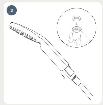
Remove the shower handle from the filter. Replace the used filter with a new one or install a dummy cartridge if unfiltered water is desired.
