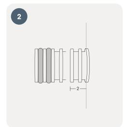
Cut the pipework connection, leaving two indents exposed from the wall. Unscrew the pipework, apply an appropriate sealing material to prevent leaks, and then securely screw it back in place.
