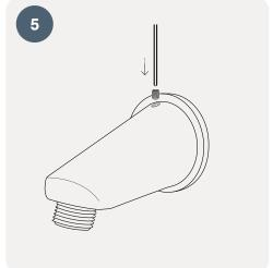
Attach the shower arm to the base plate and secure it using the grub screw.
