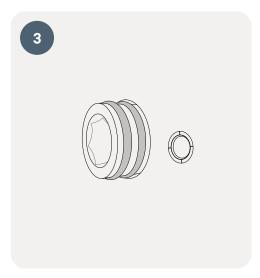
Place an O-ring onto each indent (two in total).
