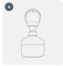
Connect the T-safe Easy-Fix Shower Filter (02-092031) or the T-safe Medical Fixed Shower Filter (02-092034) to the shower arm using the 1/2" threaded connection.
