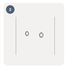
Insert the wall plugs, ensuring they are flush with the wall.
