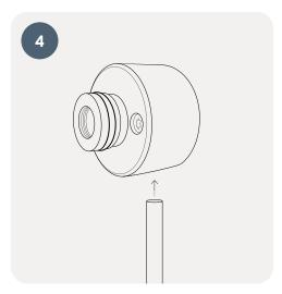
Connect the water supply pipework.
