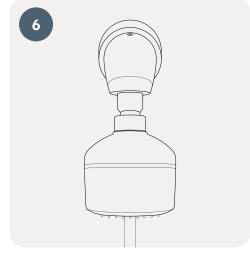
Connect the T-safe Easy-Fix Shower Filter (02-092031) or the T-safe Medical Fixed Shower Filter (02-092034) to the shower arm using the 1/2" threaded connection.
