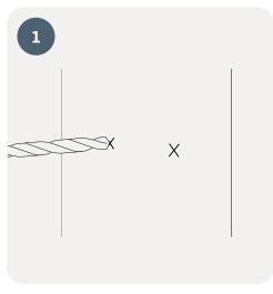
Installing the Base: Mark and drill two holes using an 8 mm drill bit.
