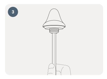
Insert the other part of the adapter and screw it in loosely by hand. Then, secure it tightly using a clean 12 mm Allen key.
