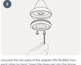
Unscrew the two parts of the adapter (90-001882) from each other by hand. Insert the base part into the Horne shower head and fasten it tightly using the original screws from the shower head and a clean 3 mm Allen key.
