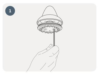
Remove the spray plate and O-ring from the Horne shower head using a 3 mm Allen Key.
