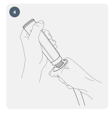
Remove the shower handle from the filter. Then, ensure the filter is firmly tightened to the hose so that no water leakage occurs.
