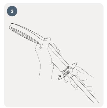
Unscrew the locking ring at the bottom of the shower filter by turning it counterclockwise by hand.
