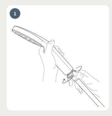
Unscrew the locking ring at the bottom of the shower filter by turning it counterclockwise by hand.
