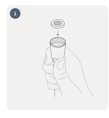
Remove the old gasket from the shower hose and insert the new gasket provided in the packaging.
