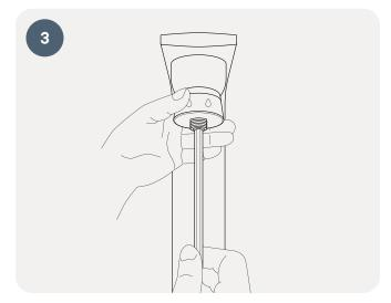
Push the adapter and the shower head ring in place and secure it with the hollow center screw using a clean 8 mm hex key. Tighten firmly.
