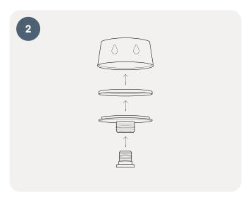
Place the transparent silicone gasket, the adapter, and the following Allen screw in the Presto shower head ring.
