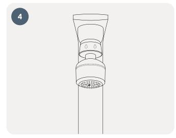
Connect the T-safe Easy-Fix Shower Filter (02-092031) or the T-safe Medical Fixed Shower Filter (02-092034) to the 1/2" thread.
