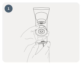
Remove the spray plate from the Presto shower head by loosening the center Allen screw.
