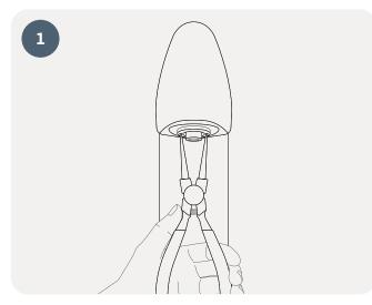
Remove the spray plate from the Delabie shower panel/head using a lock ring plier.
