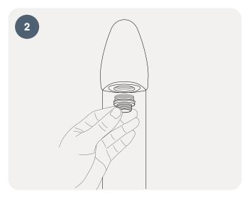
Insert the adapter into the Delabie shower panel/head by screwing it in loosely by hand.
