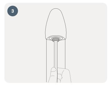
Secure it tightly using a clean Allen key.
