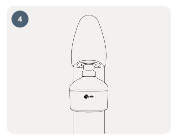
Connect the T-safe Easy-Fix Shower Filter (02-092031) or the T-safe Medical Fixed Shower Filter (02-092034) to the  $\frac{1}{2}$ " thread.
