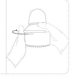
By gently turning and pulling the filter, it is easy to remove the used filter. Make sure the used filter is correctly disposed.
