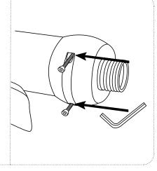
Replace the previously installed gasket in the hose conical and fasten the hose tightly to the Kitchen Spray Filter. It is now ready for use.
