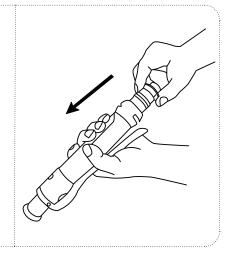
Insert the locking pawls and tighten the screws using an Allen key size 1.5 mm.
