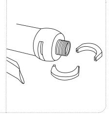
Remove the filter from the handle and dispose of the filter using normal disposal methods.
