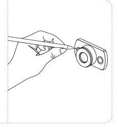
Use a Ø6 drill bit to create holes at the marked positions on the wall. Insert the provided raw plugs into these holes.
