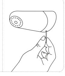
To remove the shower head, turn it counter-clockwise while simultaneously releasing and pulling it away.
