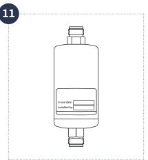
12. Re-Install filter, using replacement ½" gaskets. Ensure to orient filter correctly in the process.
