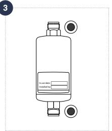
4. Tighten in-out connections.
