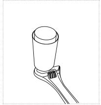
3. Remove and dispose of the used filter cartridge and pour it into a bag for disposal without contact.
