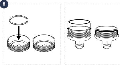
9. Install the new filter cartridge, by mounting the filter into the small outlet part.
