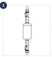
2. Open filter housing - Make sure that the outlet part is pointing up - then unscrew the small outlet part. Beware of residual water from the housing when opening the filter.
