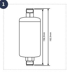
2. Ensure pre-assembled filter orientation corresponds to the flow direction in the pipe.
