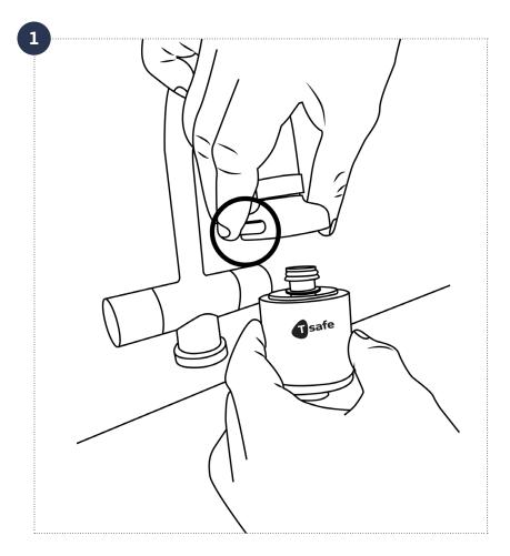
2. At the same time manoeuvre and push the tap filter inlet upwards fully into the adapter. Handle the filter using the packaging to avoid touching and contaminating the filter outlet.
