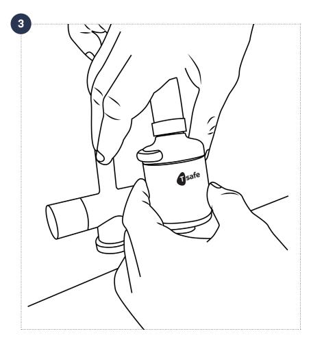
**4.** To remove the filter during exchange, press the grey locking pawl, pushing fully to release the locking mechanism and pull the filter downwards.
