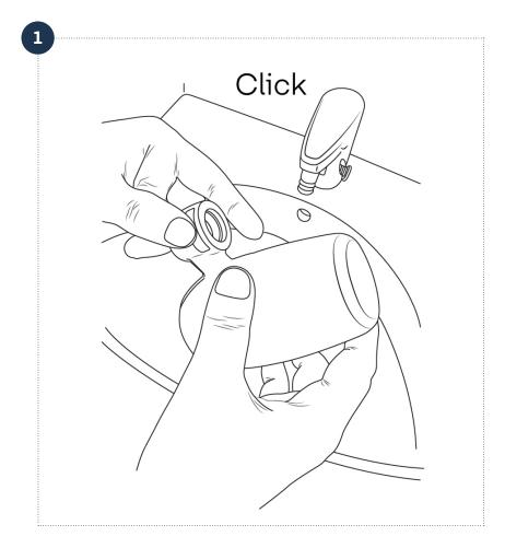
2. Push the tap filter onto the already installed adaptor. Make sure not to touch the outlet of the filter.
