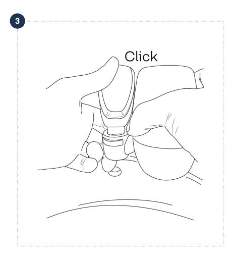
**4.** When exchanging the tap filter simply push the grey locking pawl in order to release the tap filter from the adaptor. Use a disposable bag to package the filter and discard without touching or releasing contaminated water.
