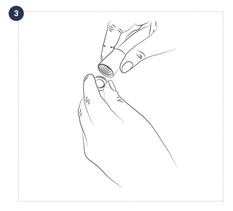
**4.** Fasten the second hose to the filter. After installation of the filter, make sure that the hoses are not twisted as to avoid reduced water flow. When the filter is installed make sure that the hoses are firmly placed as to avoid unnecessary damage of the filter.
