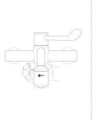
3 Demount the adapter from the tap outlet using a 10mm hex key. Clean the tap threads before refitting any inserts such as flow straighteners or aerators. ENGLISH
