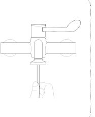
Install the product directly from the packaging and ensure that the filter does not come into contact with sources for contamination before being installed. Push the filter into the adapter until it is depressed fully with an audible 'click'. Perform a run test by opening the outlet to ensure that a watertight seal has been achieved.
